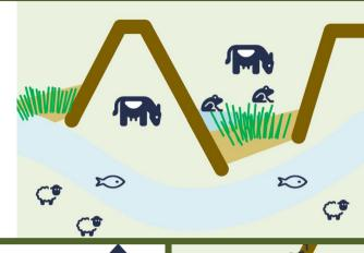
Water flowing into the bund is pushed up the valley floor, this increases the area of flood plain used and therefor stores more water, which reduces the peak flows downstream. Flood water diverted by bund
