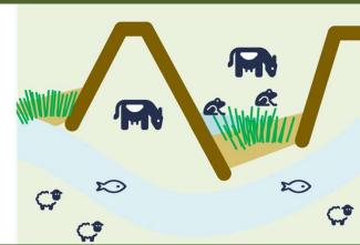
Water flowing into the bund is pushed up the valley floor, this increases the area of flood plain used and therefor stores more water, which reduces the peak flows downstream.
