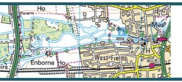
This map shows the extent of channels across the valley floor West of Newbury. These now combine into a single channel under the town bridge. A historic northern channel, has been diverted down a tiny culvert. The limited capacity of that culvert is why the northern channel reemerges in times of peak flow and floods the Northcroft area.
